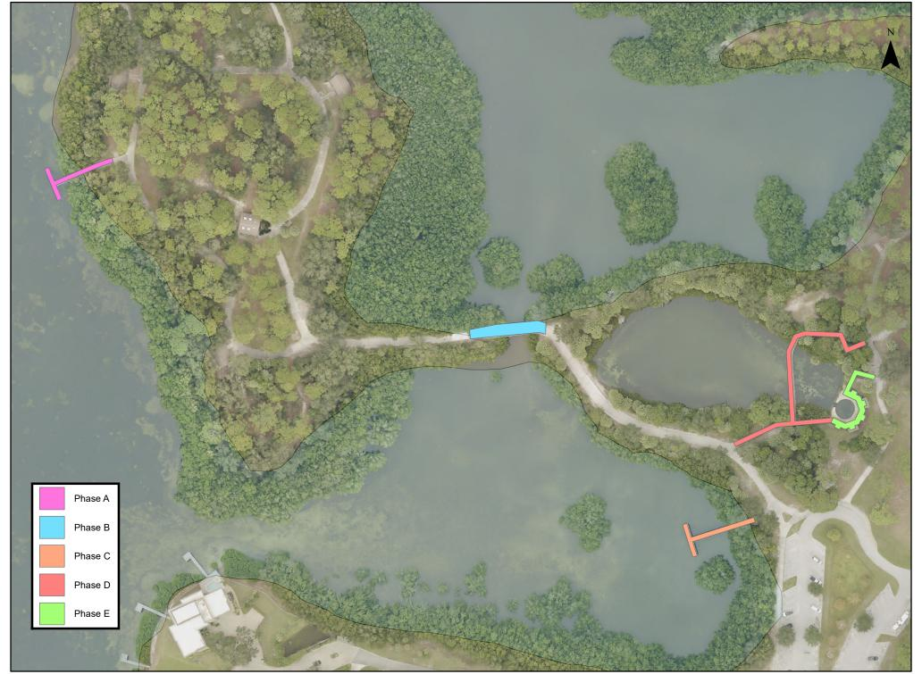
WALL SPRINGS BOARDWALK REHAB PHASING PLAN
