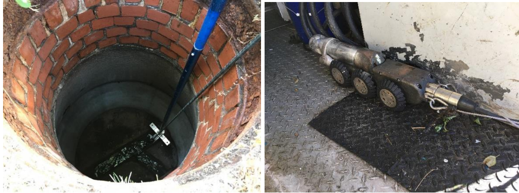
Figure 2-3. Left – Guide for camera in a manhole, Right – Camera used to inspect manholes
