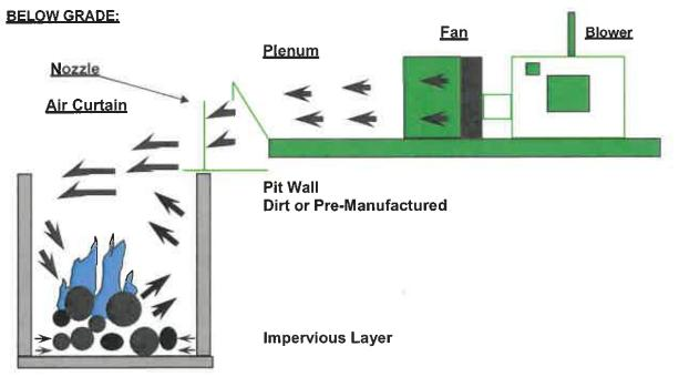
A power source, either electric motor or diesel power unit, drives a fan which in turn creates an air curtain by forcing air through a plenum and nozzle. This high velocity air travels across the top of the pit, in which a fire has been started.
