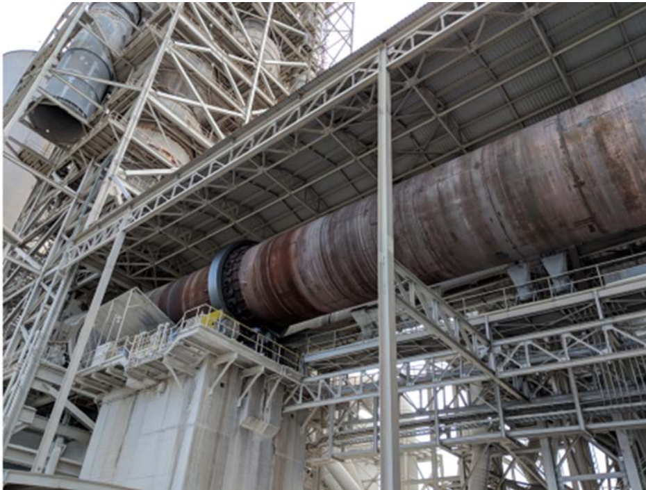
Photo 2-8 Cement kiln in South Florida where WTE bottom ash was tested as kiln feed (Photo: T Townsend)
