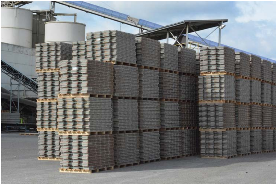
Photo 2-5 Concrete paver products in the Netherlands using WTE bottom ash as a partial aggregate replacement (Photo: T Townsend)
