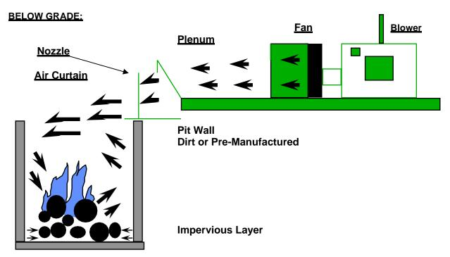
A power source, either electric motor or diesel power unit, drives a fan which in turn creates an air curtain by forcing air through a plenum and nozzle. This high velocity air travels across the top of the pit, in which a fire has been started.
