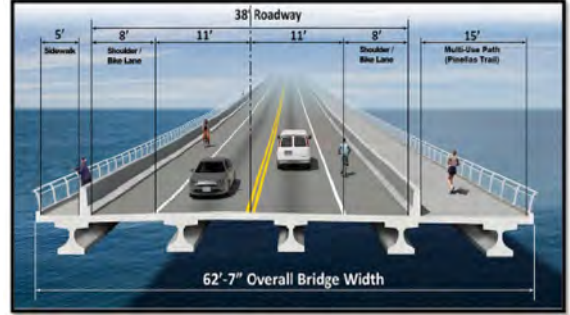
FIGURE 7-1 PREFERRED ALTERNATIVE TYPICAL SECTION (APPROACH SPANS SHOWN)
